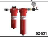
**52-531** - This unit is a point of use two (2) stage oil water extractor with a desiccant drying cartridge for one (1) gun painting operations where dry clean air is critical such as automobile or fine wood finishing. Desiccant unit has an indicator to show when unit is saturated and needs replacement. Unit comes with ball valve at inlet and regulator for one (1) gun regulation. This is what all fine finishers should have. Maximum flow is 25 SCFM and rated to one (1) micron.
