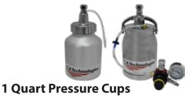
The 1qt. pressure cups are perfect for small painting jobs and are available in an aluminum or stainless steel version. Regulated versions have a one way check valve to prevent fluid from traveling back up into the gun or regulator. Pressure assist cups require a ported spray gun for operation. 10 psi max working pressure. 51-350 has a max pressure of 50 psi.
